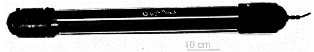
Fig. 4. Sample of pipe used in creep test under hydrostatic pressure at 180°C.
