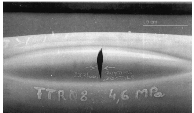
Fig. 12. Ductile failure under hydrostatic pressure (9.6 bar) at 80°C (resin A).
